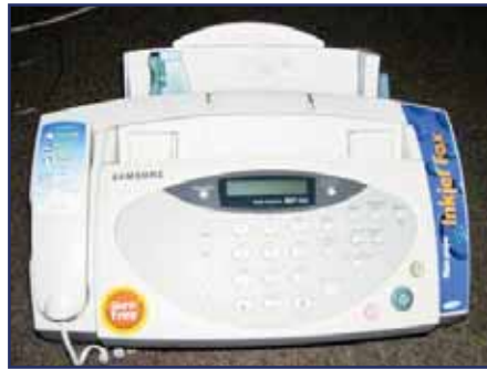
A Samsung fax machine, a model that uses ink-jet technology for output
